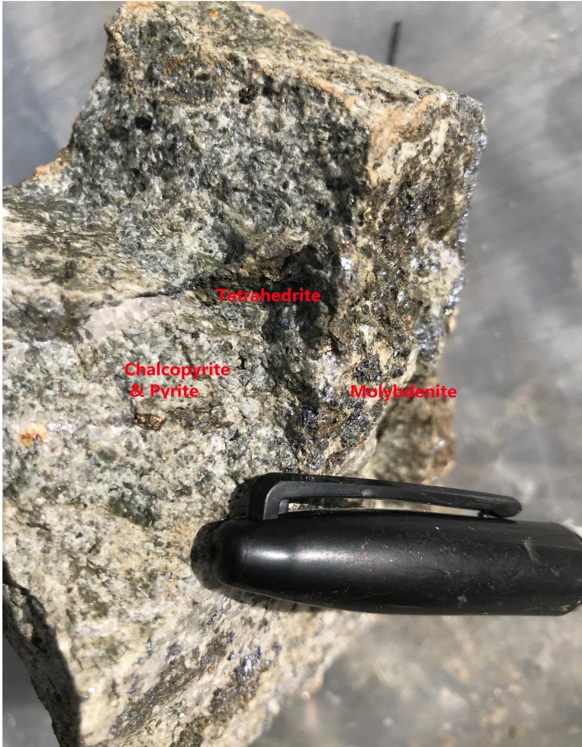
Figure 7. Granite rock sample within the contact/fault shear zone with chalcopyrite, pyrite, tetrahedrite and molybdenite minerals at NATMR006, Netalzul Mountain
