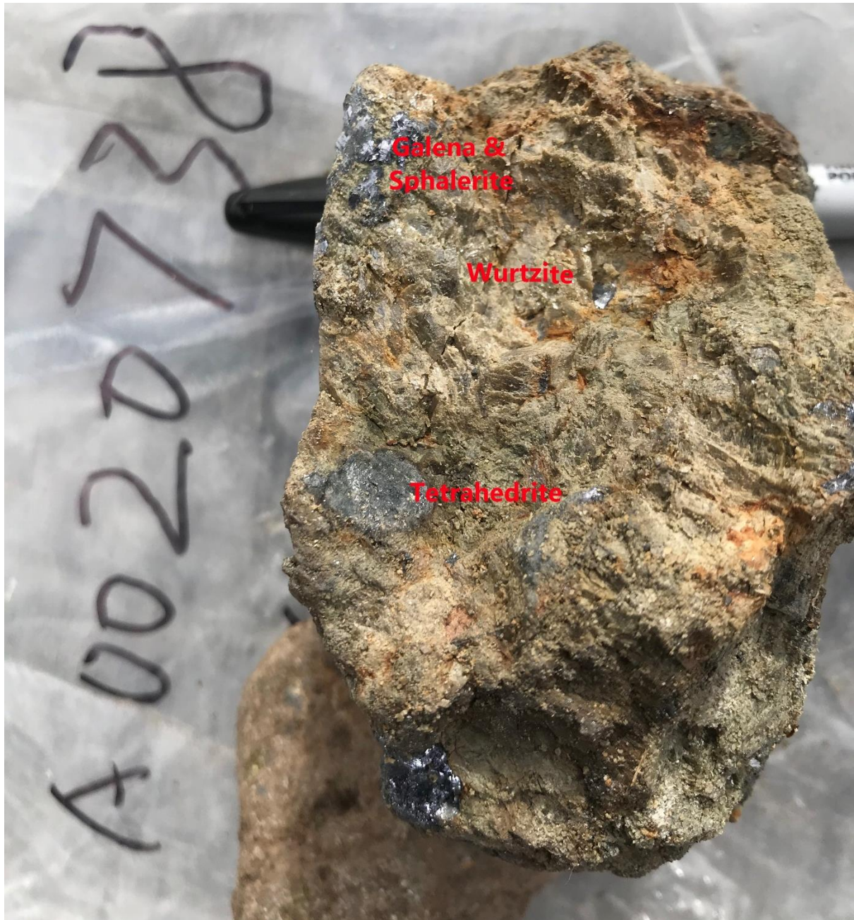
Figure 4. Rock sample from historical ore piles at artisanal workings showing massive sulfide minerals (galena, sphalerite, wurtzite and tetrahedrite) at NATMR006, Netalzul Mountain
