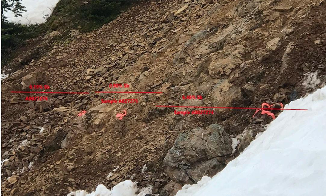
Figure 2. Chip samples taken from across six metres at KS zone 2 outcrop at Kispiox Mountain Project.
